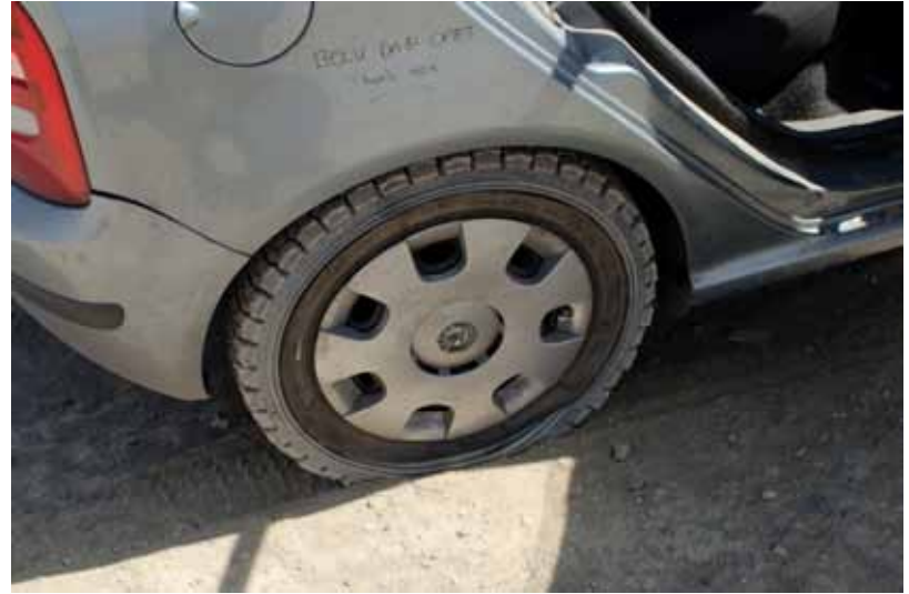
First flat tyre. Tyres larger than spec for the car plus overloaded rear suspension meant that the back tyres hit the wheel arches on bumpy roads, destroying them.
