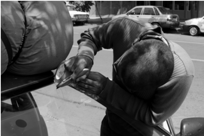
Windscreen repair – taping over the crack.
